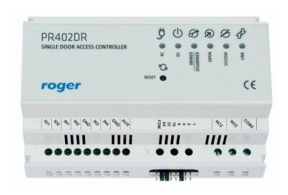
PR402DR access controllers may operate as standalone access control units or in integrated access control system with CPR32-SE network controller. In standalone mode PR402DR autonomously supervise two-way door passage and do not need to communicate with PC nor any other equipment, events are registered in their internal buffer and time related functions are managed by
