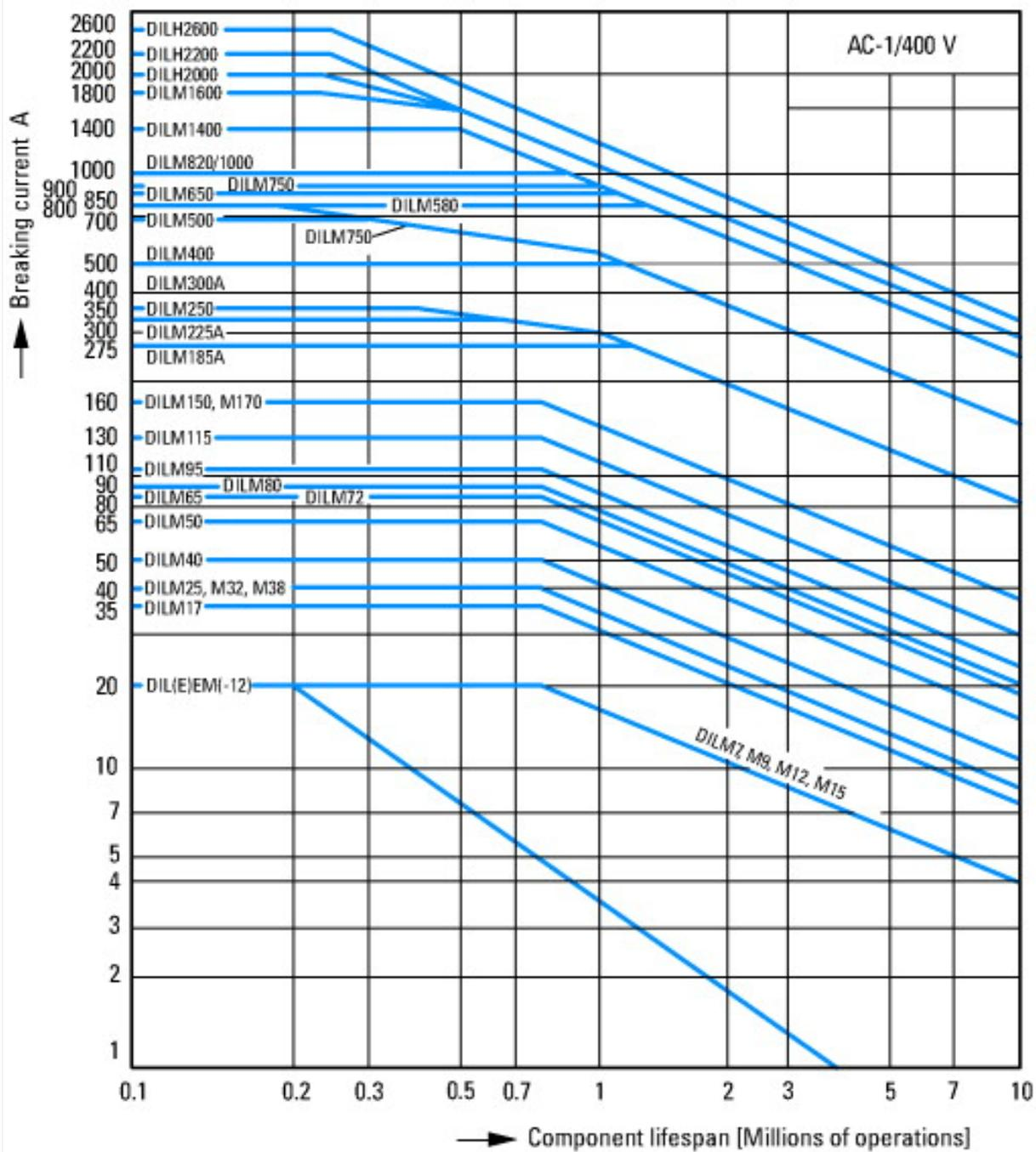
Switching duty for non-motor loads, 3-pole, 4-pole
