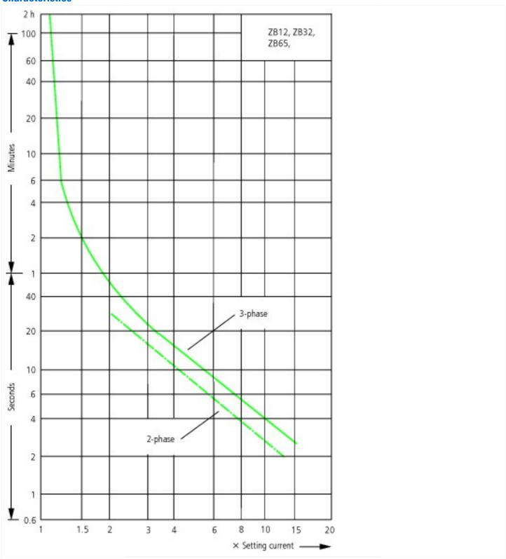
These tripping characteristics are mean values of the spread at 20 °C ambient temperature in a cold state. Tripping time depends on response current. On devices at operating temperature the tripping time of the overload relay drops to approx. 25 % of the read value. Specific characteristics for each individual setting range can be found in the manual.
