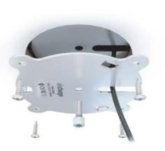
2. Secure the charger to the work surface with the steel plate provided, using the appropriate length bolt (use 16mm bolt for standard 1" desk) - use wood screws for extra security
