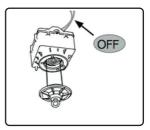
Be sure to turn off the power during installation. Install only when de-energized.
