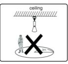
During installation and operation, staying under the load within a radius of 3 m is prohibited.
