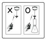
Do not operate the system without a weight on the load plate. The weight information on the type plate must be observed.
