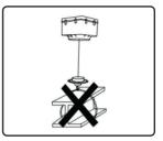
Lighting lifts must not be used to raise or lower objects that are not specified by the manufacturer.
