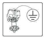
Make sure the device is properly grounded.
