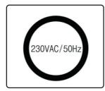
Use the correct power source indicated on the rating plate, otherwise a system failure may occur.
