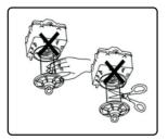
Do not place limbs or objects between the top and bottom contacts during operation as this may result in personal injury and/or system failure.
