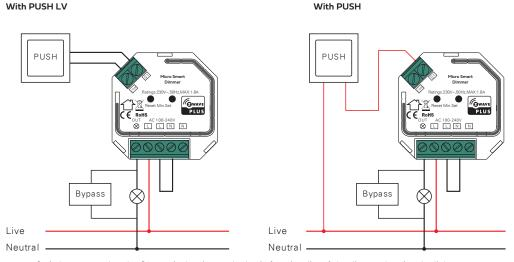
**NOTE:** Switch connected to the S1 terminal activates the basic functionality of the dimmer (turning the light on/off, dimming).
