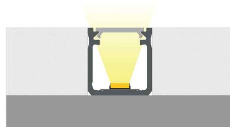
The end result of installation of groove mounted profile Y with BASIC cover between the boards
