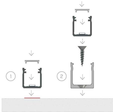
Installation instructions for profile Y with a BASIC cover using [1] double-sided tape, [2] a mounting clip and screw
