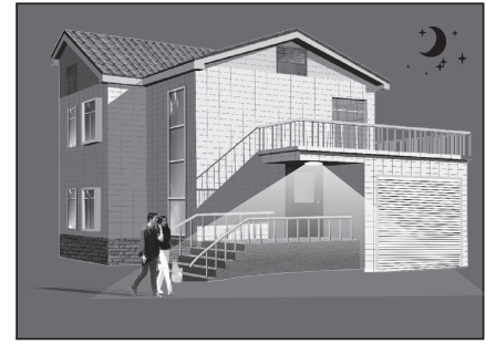
With insufficient ambient light, the sensor switches on the lamp when motion is detected.
