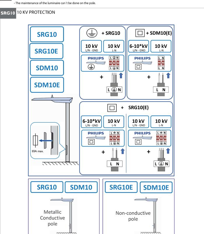
\* 10kV for L/N – GND non-conductive connection
