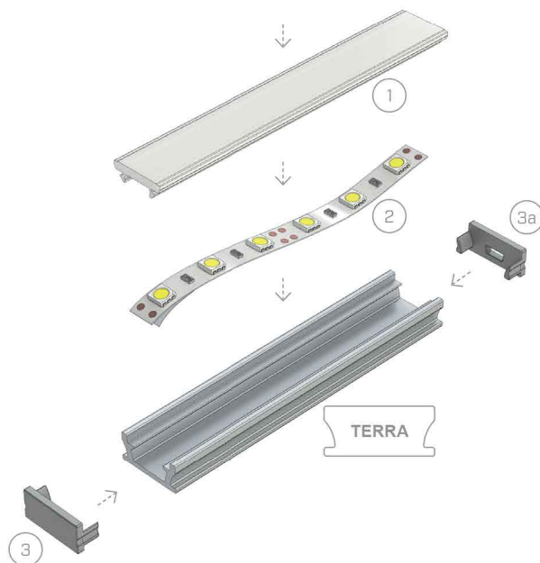
Assembly scheme for the elements of the lighting system using TERRA profile and (1) a floor cover, (2) LED strip, (3) end cap without hole (3a) end cap with hole
