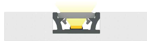
The end result of installing a TERRA profile with a floor cover
