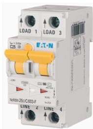
**electronic residual current circuit-breaker/miniature circuit-breaker, 25A, 30mA, miniature circuit-breaker trip curve: C, 2pole, residual current circuit-breaker trip characteristic: F**
